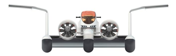
2. The craft design solution includes shock-absorbing balloon tyres under the wing collars and the centerplane. This gear provides more comfort during cruising on the wavy water. Moreover, the combination of the balloon tyres and air-feeding propulsion provides the amphibiousness of the craft (ability to move to the flat shore without any infrastructure required).
